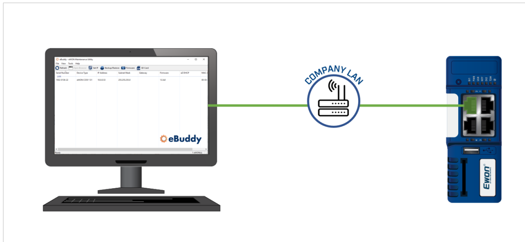
Fig. 21 Connect the computer indirectly to the Ewon though Company LAN
