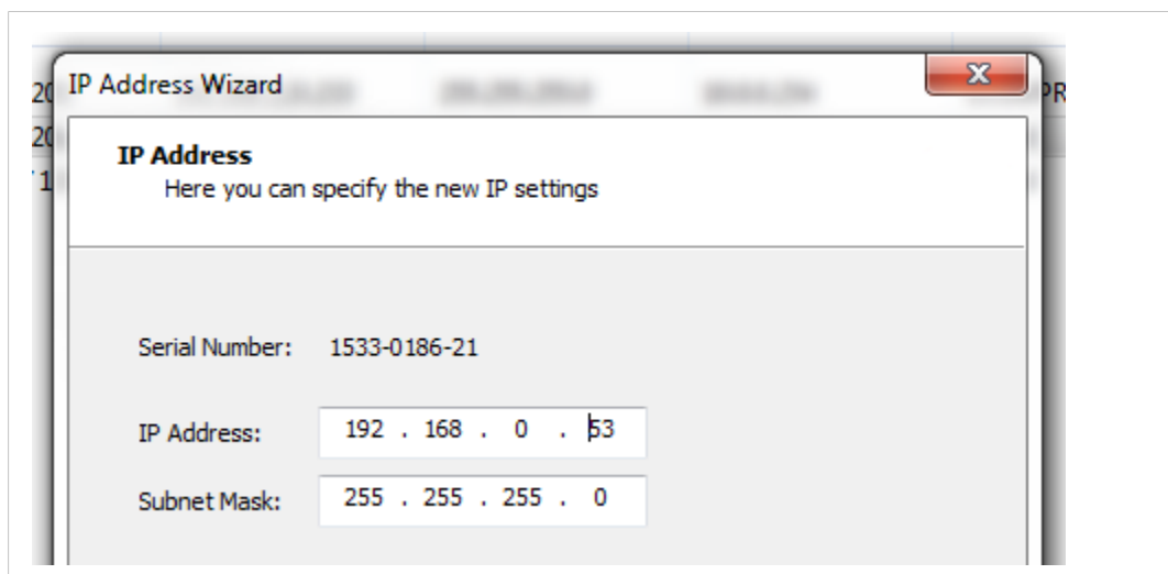
Fig. 26 eBuddy — LAN IP address and Subnet mask
