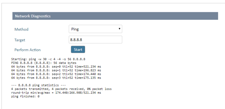
Figure 29. Example, Ping response message from Target 8.8.8.8
