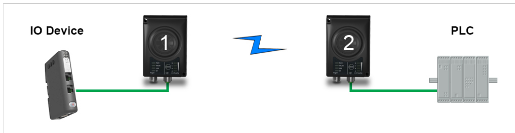
Fig. 21 EtherNet/IP wireless network
