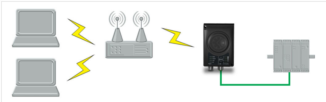
Fig. 23 Adding WLAN connectivity
