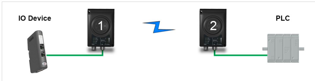
Fig. 20 PROFINET wireless network
