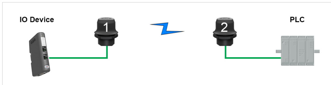
Fig. 23 EtherNet/IP wireless network
