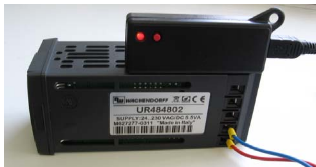
Figure 3: Inserting Programming module on UR4848xx
