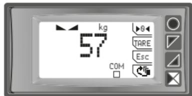
These functions, enabled by the relevant parameters during configuration, allow to reset the measure or to switch from gross to net weight and viceversa. This window can be entered by process visualization, pressing one of the function keys.
