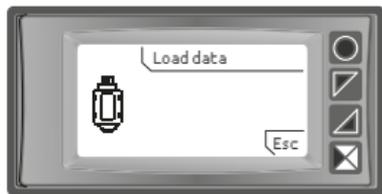
The user can either "Load data" load the parameters from the memory card or "Esc" cancel the operation without modifying the current configuration.
