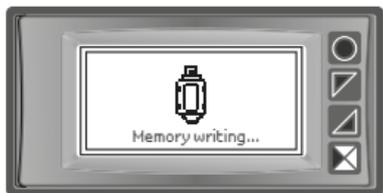
Saving is signalled by a message on the display.
