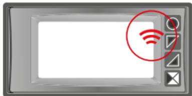
Position of the NFC/RFid antenna for communication with smartphone and reading / writing of data.
