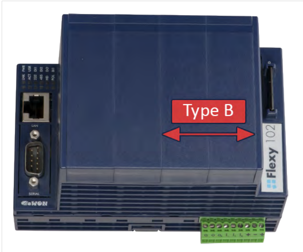
Fig. 5 Position of the “B” Slots on a Flexy 10x & 20x.
