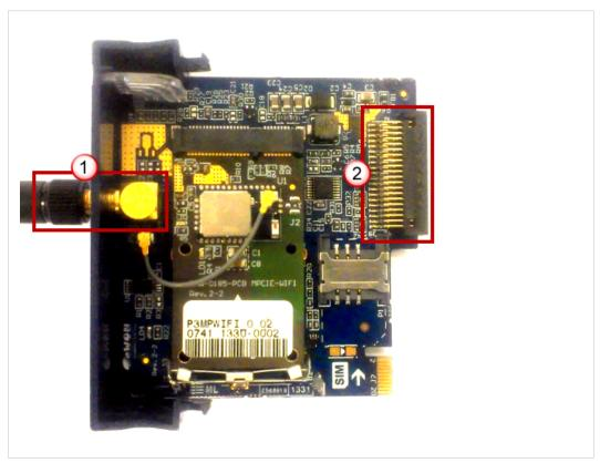
Fig. 1 Mechanical layout and interfaces
