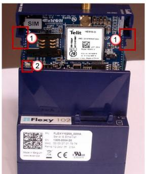
Fig. 6 Remove the slot fillers
