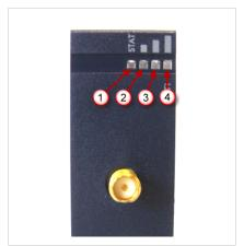
Fig. 3 Front panel LEDs
