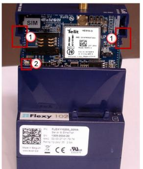
Fig. 6 Remove the slot fillers
