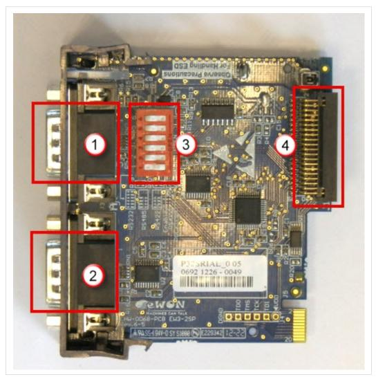
Fig. 1 Mechanical layout and interfaces
